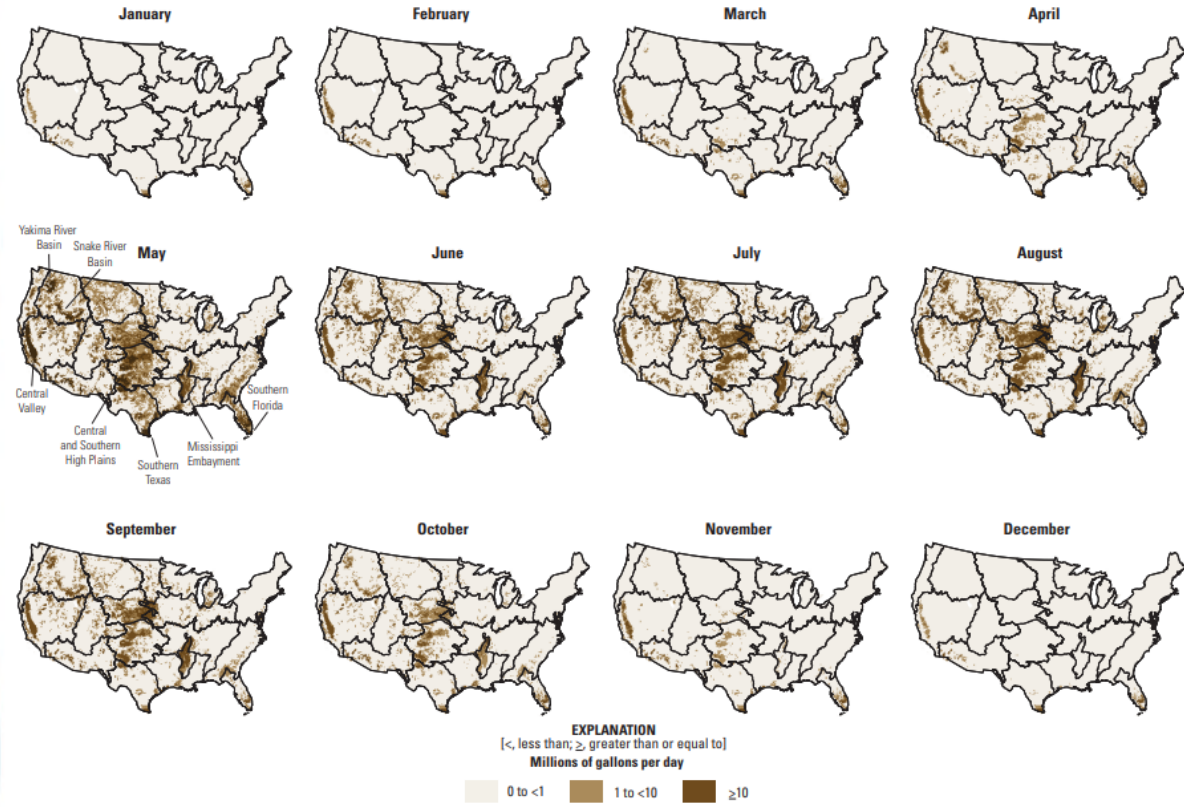
Figure 13. Model estimates of crop-irrigation water withdrawals by month by 12-digit hydrologic unit codes (HUC12s) for the conterminous United States, averaged for water years 2010–20. Black lines indicate hydrologic region boundaries. Model estimates for crop-irrigation water withdrawals are from Haynes and others (2024).
