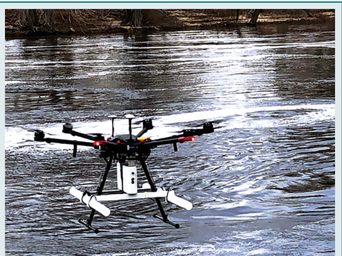
Mapping river-water depth by using a drone-mounted ground-penetrating radar system (white equipment). Photograph by John Lane, U.S. Geological Survey.
