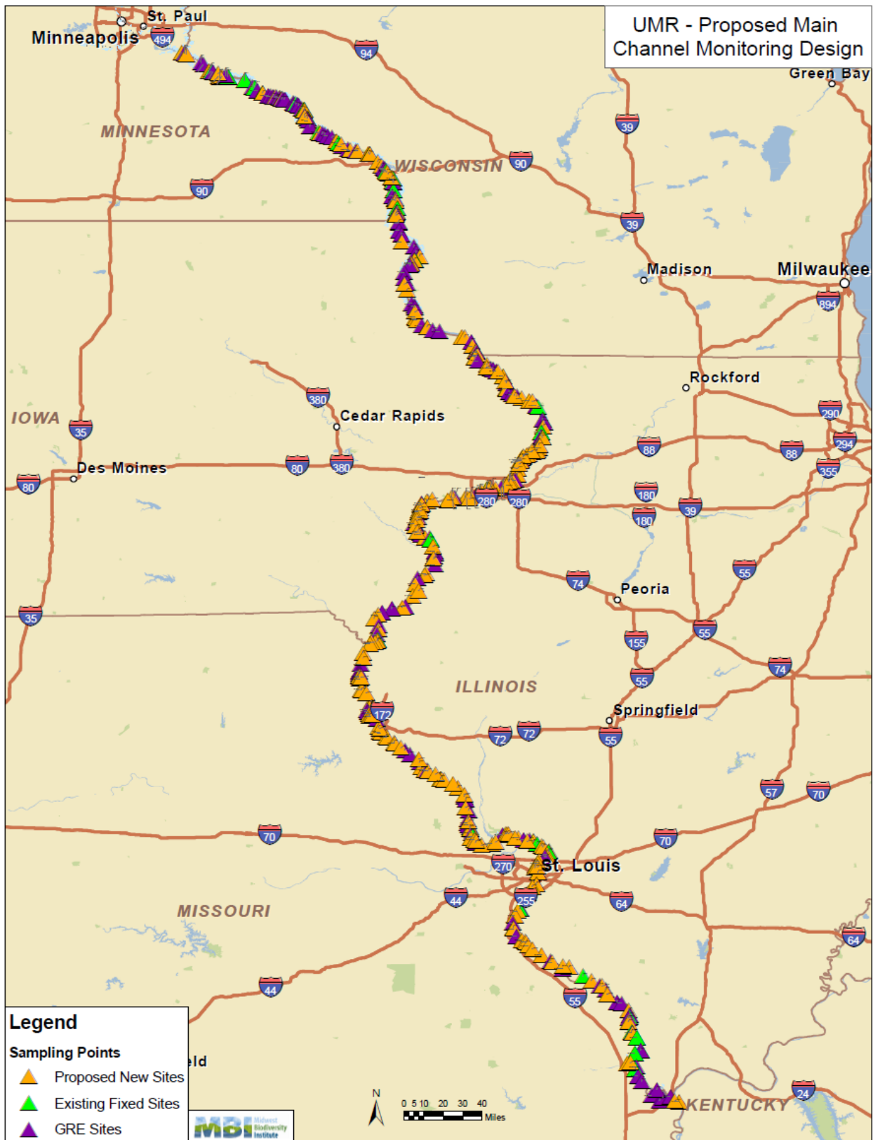
Figure 4. Intensive Pollution Survey design option sites based on site location methodology and also including 2004-6 GRE and existing fixed station sites as a part of the design and to show a comparison of site density. This includes main channel and side channel sites.
