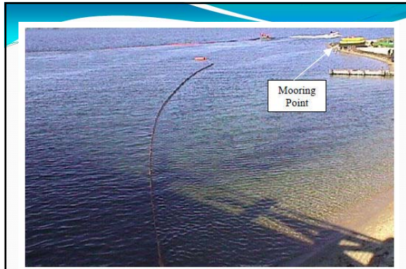
Figure 5-10. Boom vane deployed in Martha's Vineyard. (Mooring line is attached to point of land in upper right-hand part of picture)
